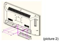
4. Use 4 screws to fix the TV on the wall mount bracket .Please find there are 4 VESA holes on the back of the unit (Refer picture 3).
